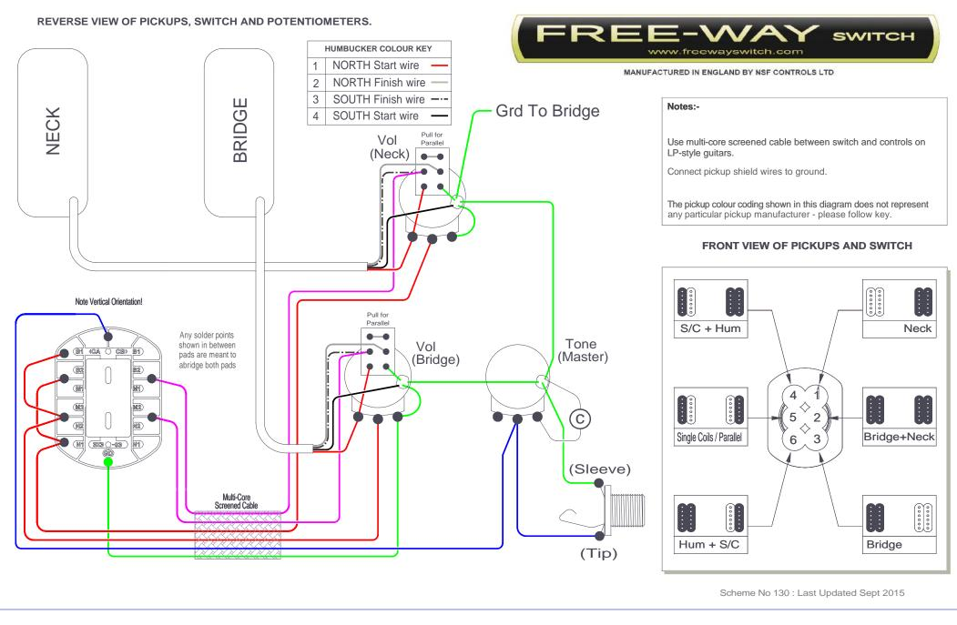
Model Not- 3X3-03 Free-Way Switch HH Hum + S/Coil Combinations + Parallel 2V/1T
