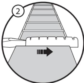
STEP 2. If the nut is not sitting in a slot, usually a light tap with a small block will set it free. If it is sitting in a slot, gently tap it out sideways using a hammer and a screw driver.
