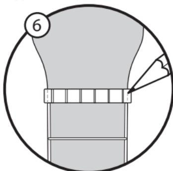
STEP 6. Once you've done the thickness and the height, you just need to sand the ends of the nut so that they are flush with the neck. Just use a pencil and mark the ends of the nut that are sticking out, remove it from the neck and sand it to your marks.
