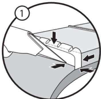
STEP 1. Remove the strings. Trace around (score) every edge of the nut with an exacto knife to prevent lacquer sticking to the nut and the neck and chipping away.
