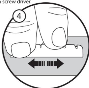
STEP 4. See if the Graph Tech nut fits into the slot, without forcing it. If it's too thick, place a 400 to 600 grit sand paper face up on a flat surface and sand down the sides of the nut until it fits in the slot snugly but is easily removable.
