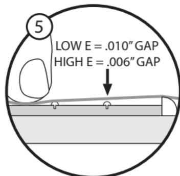
STEP 5. Restring the high and low E strings and tune to pitch to check for correct height. Pushing down on the third note of the low E string should result in a .010" gap between the string and the first fret; high E string should be .006"
