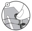
**Pull up on the string** to slide the ball end up the bridge pin and anchor it against the bridge plate, then **push the pin down** into the tapered hole. The pin does not have to be tight to hold the string firmly. Push gently to seat the pin.
