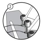
**Remove your old bridge pins** using your fingers or a pin puller like the one on the end of most string winders.
