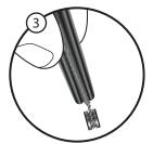
Align the string with the groove in the bridge pin, and let the ball end extend beyond the end of the pin. Insert the ball end and the bridge pin half way into the tapered hole in the bridge.
